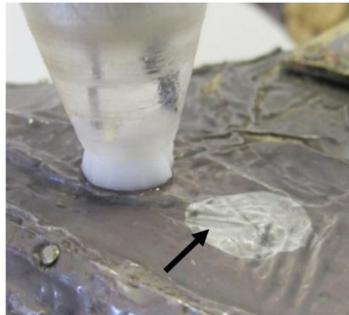
**Fig. 6:** Detailed view of a cleaned spot (black arrow) and reduction in progress with the PLECO. ©Abbaye Saint-Maurice
