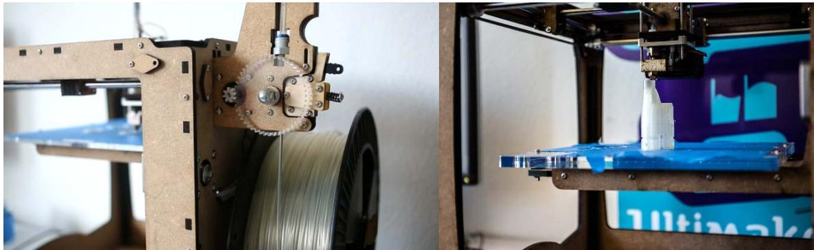
*Fig.1: View of the Ultimaker®: a 3D printer used for the manufacturing of the PLECO. ©FabLab-Neuch*
