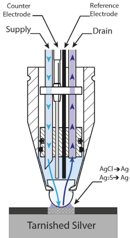
**Fig. 5:** Sectional view of the PLECO electrolytic cells. ©HE-Arc CR
